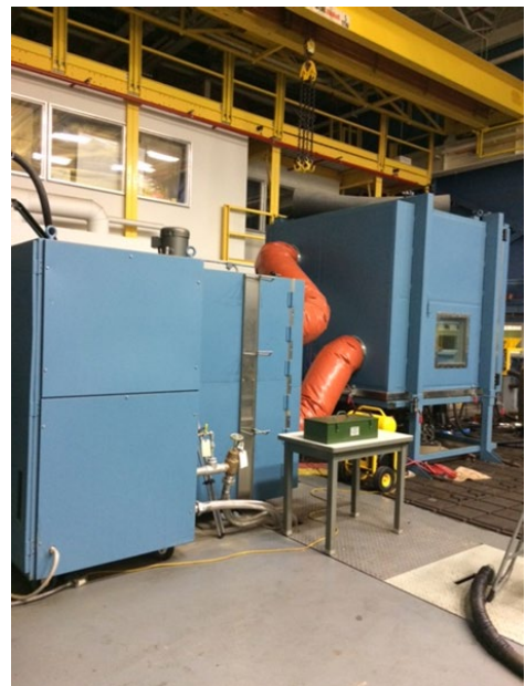
MAST Chamber for MIL – STD – 810G
