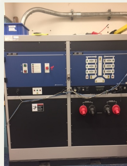
Power Cycling Station
