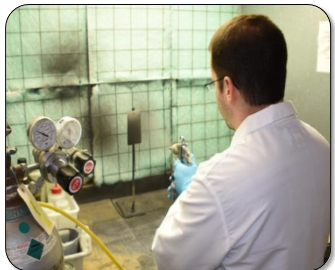
GSPF Research Engineer preparing steel panels for solid film lubricant testing.
