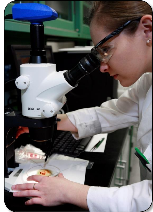
GSPF Chemical Engineer examining particulate contamination in fuel.
