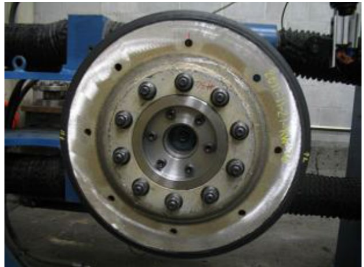
Road Wheel Durability Testing
