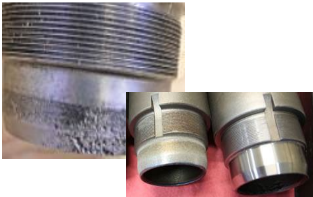
Abrams Road arm before repair (L) and after repair (R).
