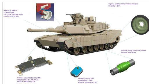
Track and running gear components that the Elastomers Lab analyzes and re-engineers to improve the component durability and system readiness.
