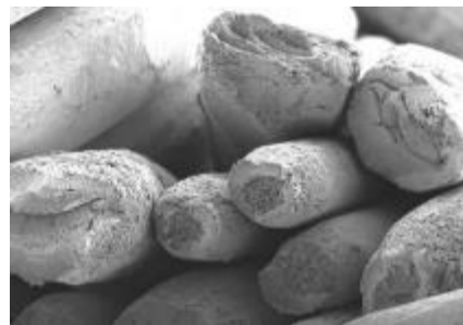
Individual steel cable braids (electron microscope)
