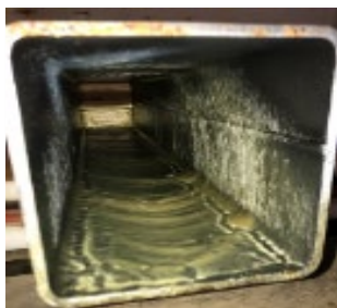
Specimen protected by cavity wax during corrosion testing
