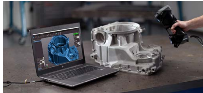
3D Laser Surface Scanning
