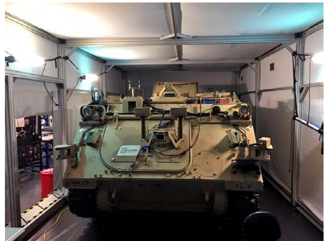
M113 Inside RF Shielded Enclosure
