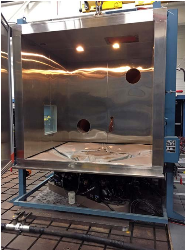
MAST with environmental chamber
