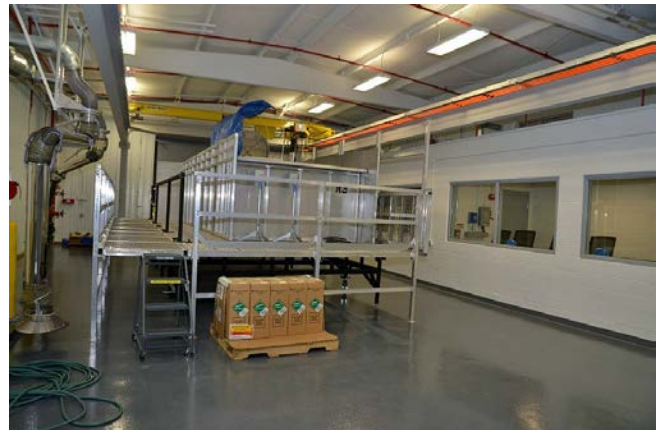
FP TIL reconfigurable chamber, used for fire protection research and vehicle integration testing
