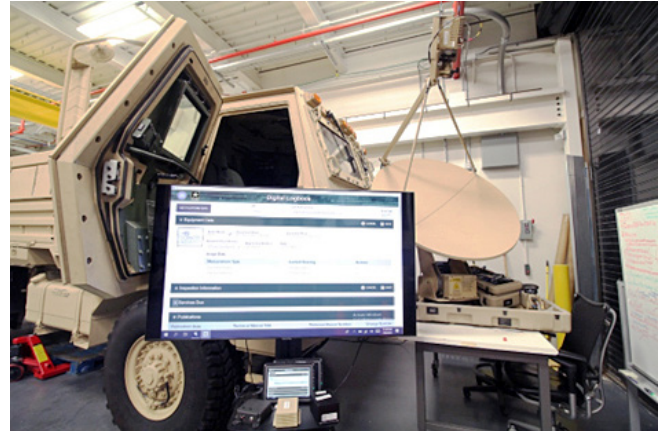
The PL SIL's M1083 A1P2, a DLB tablet, vehicle data collectors, and spare CSS VSAT
