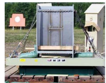
Target Setup for Weld Evaluation Testing
