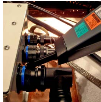
Electrostatic Discharge Testing
