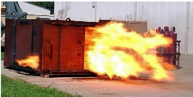
Fireball Generator: The Fireball Generator creates and ignites a pressurized, heated fuel spray to simulate a ballistic event where a threat has penetrated a vehicle's fuel tank.
