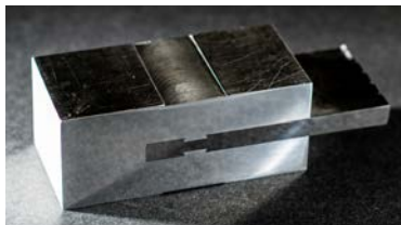
Dissimilar Material Joining Steel to Aluminum and Aluminum to aluminum (Different series)
