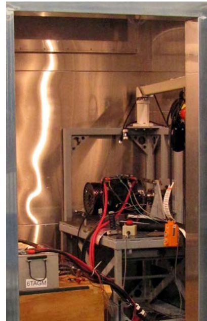
Alternator Test Inside Environmental Chamber
