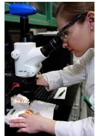
F&L Chemical Engineer examining particulate contamination in fuel.
