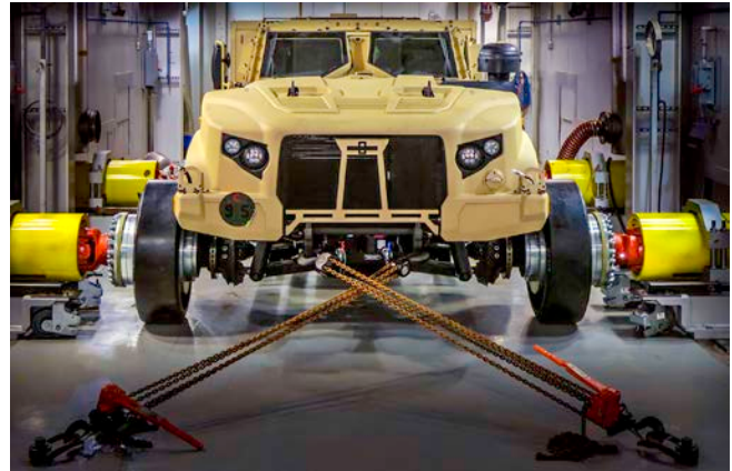
PEVEL - JLTV (Full Load Cooling Test)
