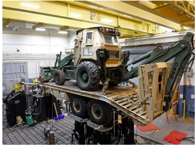
PMBS with test trailer and mission payload
