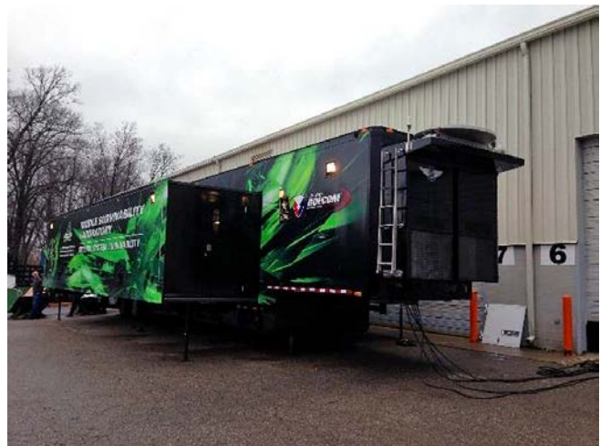
GVSP Test Trailer expands on both sides providing a large work area. Additional secure room in the goose-neck for sensitive material.
