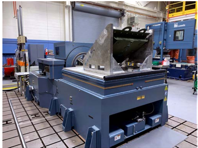
T5500 ED shaker with test component
