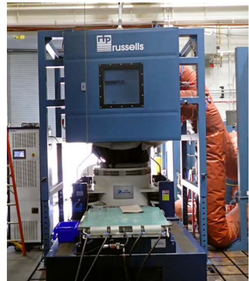
ETS 748 ED Shaker with Environmental Chamber
