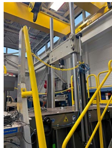
Empty Load Frame
