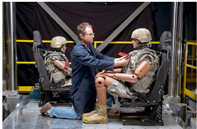
Readying ATDs on the CCUBS Platform in Preparation for a Test
