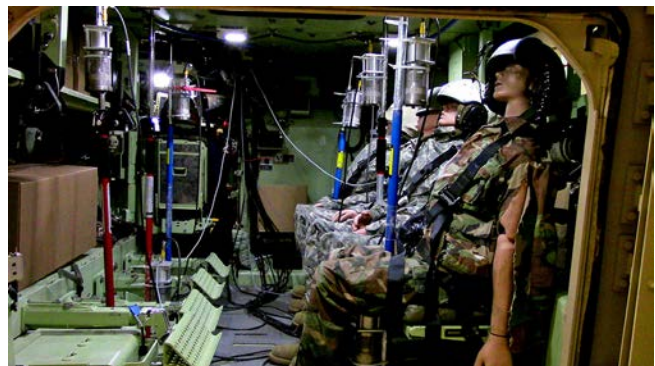
Agent Concentration Test: System installed in the Reconfigurable Fire Box. Sensors are mounted to monitor agent dispersion.
