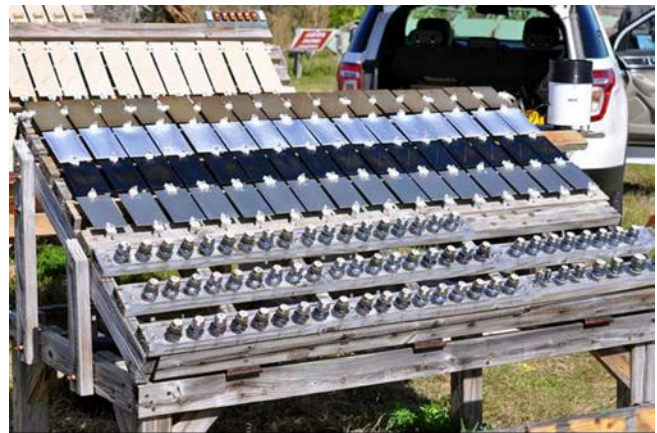
Outdoor Exposure Testing of Cadmium-Free Electrical Connectors
